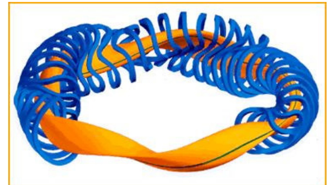
Modular coils: W7-X (Germany-under construction)
